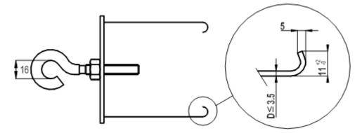
Figure 8 – Fastening device for elbow separable connectors
