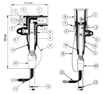
Note: maximum width (215 mm) allowed for elbow connectors, may be referred according to the design to the edge of the fastening device (as in the figure) or to the edge of the protection cap of the capacitive socket.
