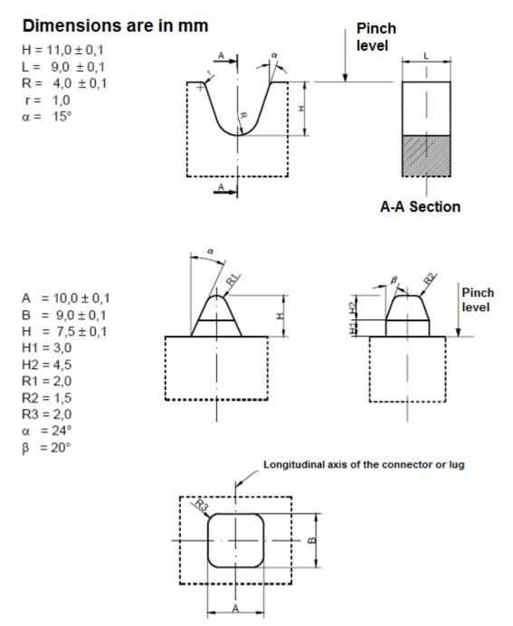
Figure 6 – Tool for compressing the earthing lug
