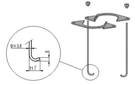
Figure 9 - Fastening device for straight separable connectors
