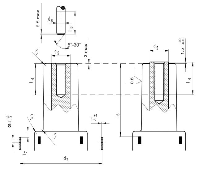
Figure 5 – Contact and fastening device dimensions (mm)
